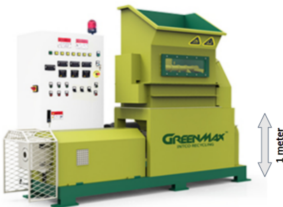
Figure 1. A typical industrial EPS densifier, which uses high temperatures and mechanical screws to simultaneously melt and crush clean EPS into large billets for recycling.
