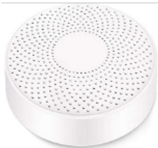
Figure 17. “FULOXTECH” (USB plug-in). Rated ozone production: 2 mg/hr. Source: amazon.com. For performance, see Figure: 9.
