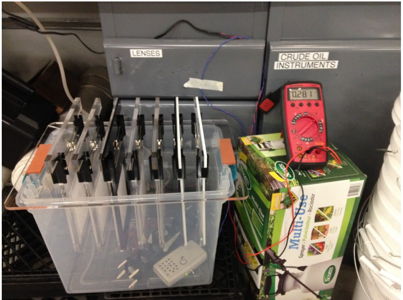
Figure 1. Samples of filter material being exposed at controlled ozone concentration in an improvised ozone disinfection chamber.
