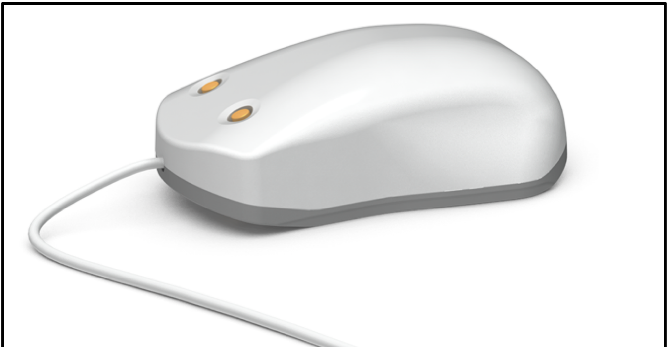
Figure 1. Vibrotactile stimulator device. Yellow tips represent stimulation sites and feedback buttons. Digits are stimulated as the yellow tips vibrate, and subjects are able to provide feedback by pressing on the yellow tips. (The Brain Gauge; Cortical Metrics; Carrboro, NC).
